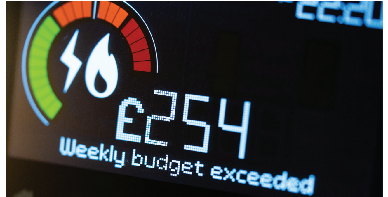
Figure 9: Smart meter with budget exceeded warning
